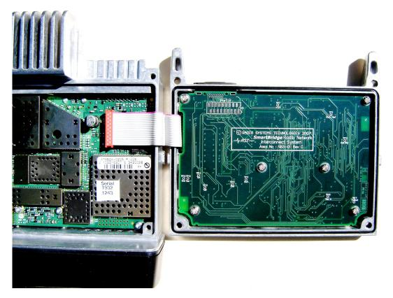
Smartbridge® is fully compatible with most standard Trunked and Conventional radios. Popular choices for the Trunked radios are the Tait TM8200 series for MPT1327 applications, and Motorola radios for SmartZone (MCS2000 and XTL1500/5000 series), TETRA (Motorola TMT500) and LTR versions (GM338 and similar).
